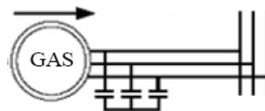
Figure II| Squirrel cage Induction Generator directly connected (fixe speed)
