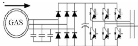
Figure III| Squirrel cage Induction Generator with a Power Converter link (variable speed)
