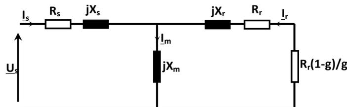
Figure IX | Induction generator steady-state model
