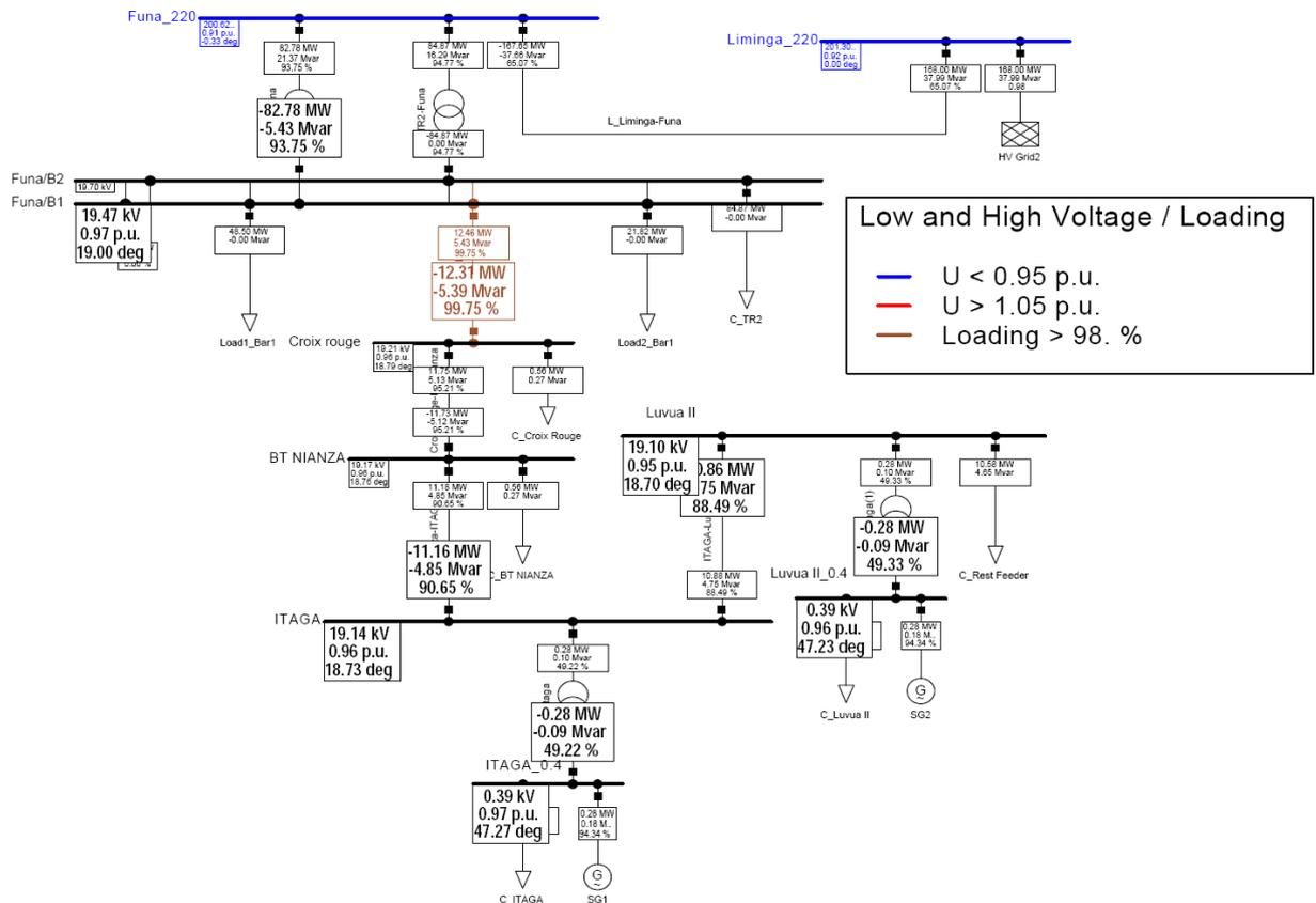
Figure XIII | Simulation #4 – Load flow results on the single line diagram of the grid after integration of synchronous generators.
