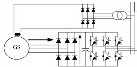
Figure I| Synchronous Generator with a Power Converter link
