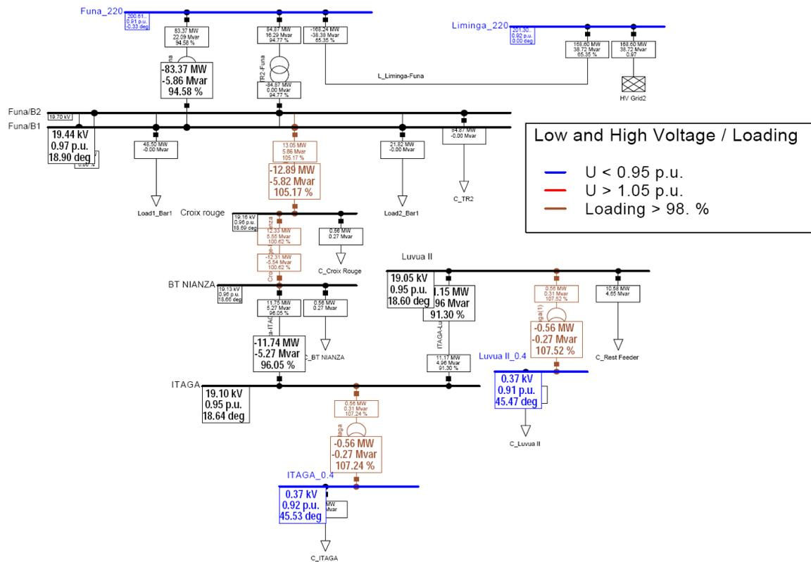
**Figure XI | Simulation #1 – Load flow results on the single line diagram of the grid during initial situation**
