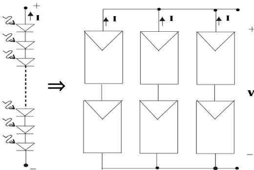
Figure V | Photovoltaic array
