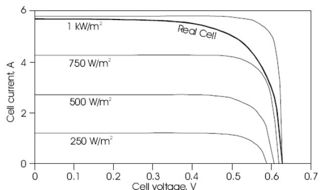
Figure VII | I-V characteristics of real and ideal PV cells [Messenger et al, 2005]
