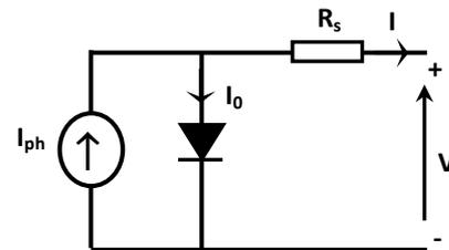
Figure VI | Photovoltaic cell model
