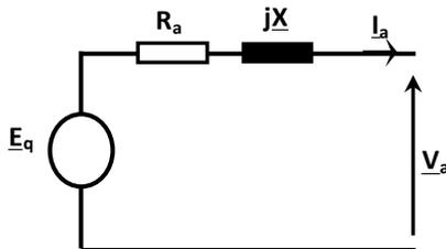
Figure VIII | Synchronous generator steady-state model
